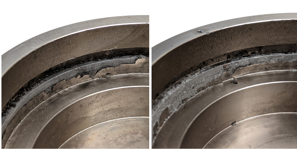
(a) Sublimation cup right after disassembly (b) Sublimation cup after a few days at room conditions.
